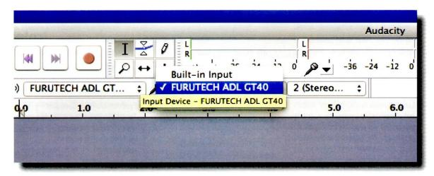
It is important to set Audacity to see the computer's inputs and outputs, to avoid silence. This is done in the top bar where external devices will identify themselves over USB: here you can clearly see the Furutech has declared its presence to the Mac and to Audacity. Don't forget to go to Sound in the Mac's System Preferences and set its Input and Output to the external source too.
