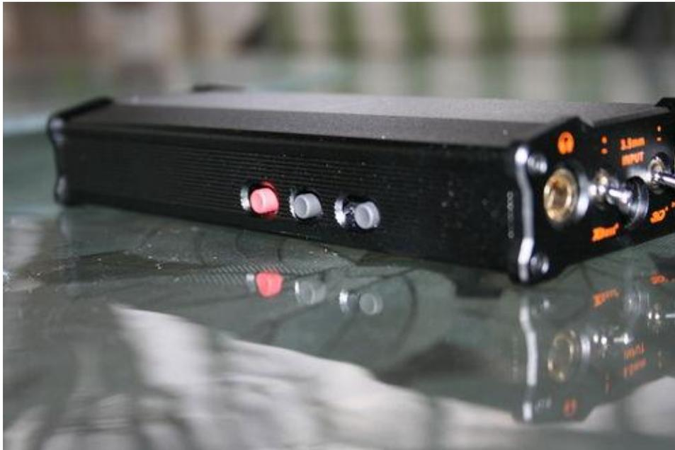
Towards the back of the unit we find a two position switch indicating Preamplifier and Direct mode. Direct mode is used as a fixed RCA output that bypasses pretty much everything else on the unit and goes straight to your power amp, headphone amp, etc.
