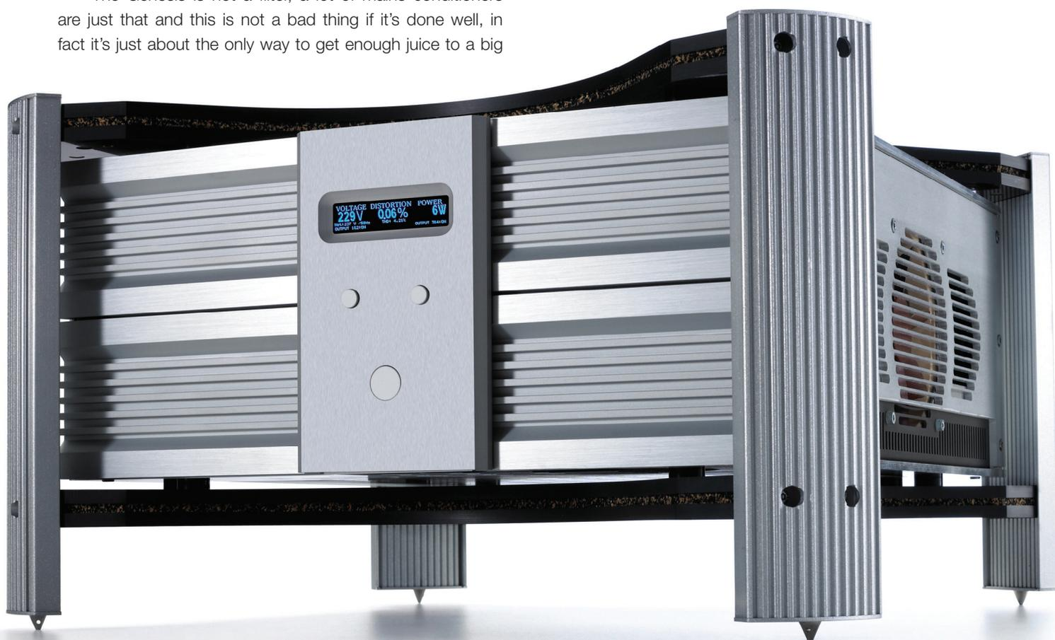
► mains by imposing a template frequency on it (50Hz in the UK) as that approach doesn't remove distortion. Instead it builds a completely new sine wave at the desired frequency, which is then amplified and delivered via transformers with copper foil between primary and secondary outputs to stop any noise and distortion getting through. It's designed to dramatically cut harmonic distortion (THD) on the mains.
