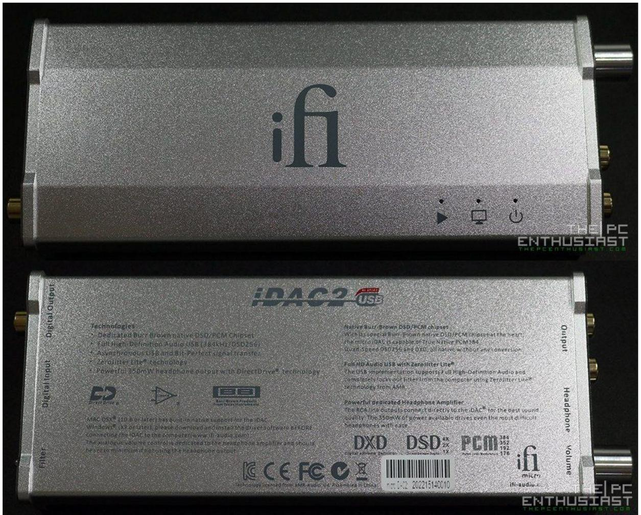
Above you see the top and bottom view of the micro iDAC2. The enclosure is pretty much standard design of an iFi portable device. On the top portion, there are three tiny holes with their respective labels. The play or arrow indicator changes color depending on the audio format that you are feeding the iDAC2. The LED colors are as follows: Green - 44/48 kHz, Yellow - 88/96kHz, Cyan 176/192 kHz, White DXD352/384 kHz, Blue - DSD2.8/3.1 MHz, and Magenta DSD5.6/6.2/11.2/12.2MHz.
